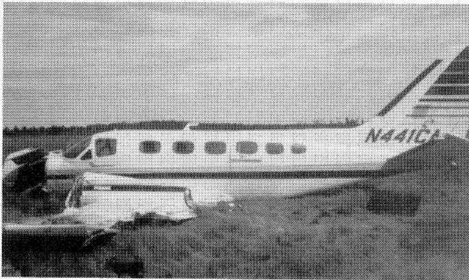
The Cessna Conquest after an encounter with seagulls during take-off from Fort Frances, Ontario.
